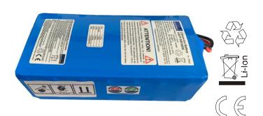
Lithium-Battery Pack with protection electronics (PCM single cells monitoring), protects the battery against overcharge, deep discharge, short circuit, Implemented cell balancing, and Gas Gauge with SMBus Interface.
